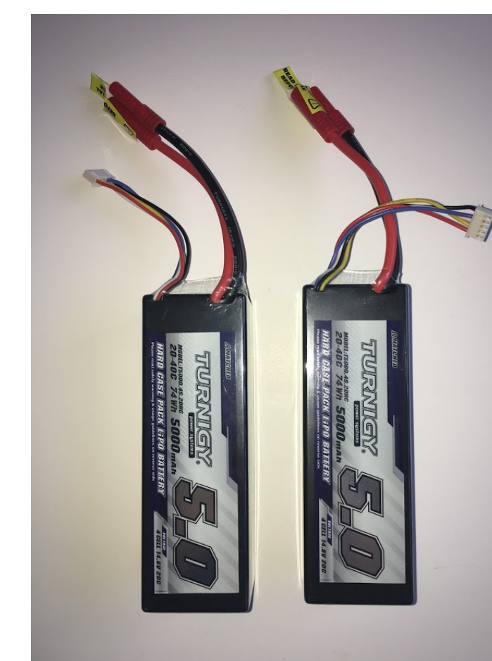
Figure 6: Turnigy 4S 5000 mAh LiPo hard case battery packs
