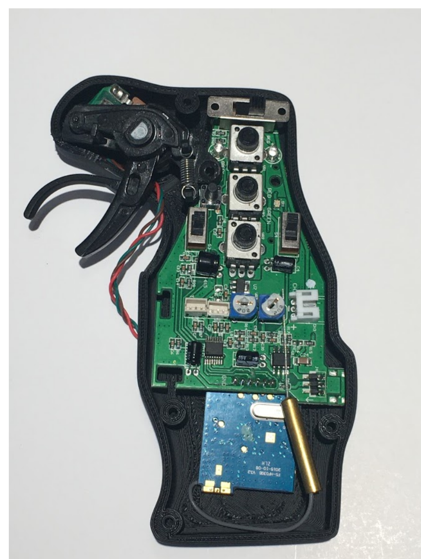
Figure 2: RC components assembled into newly constructed housing
