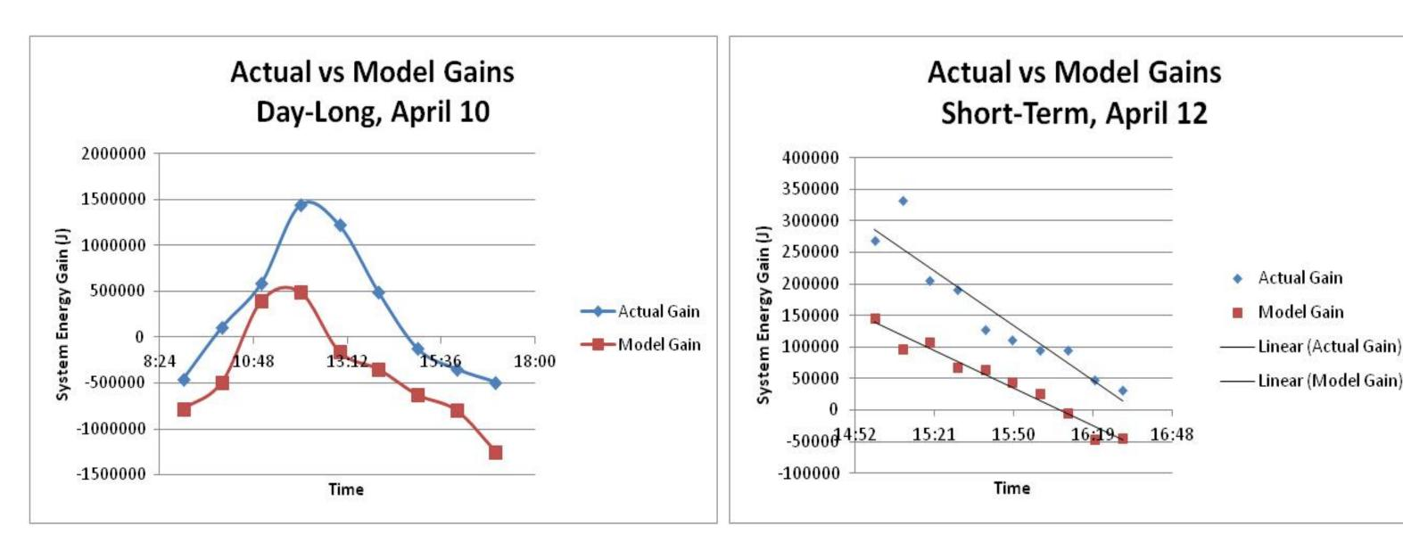
Due to the nature of the data, the difference between the actual and model predicted energy gain was a better basis of analysis than percent error. Three Short-Term tests were performed and the differential energy gain error is shown in the top left plot below. The errors are scattered and decrease with time of day.
