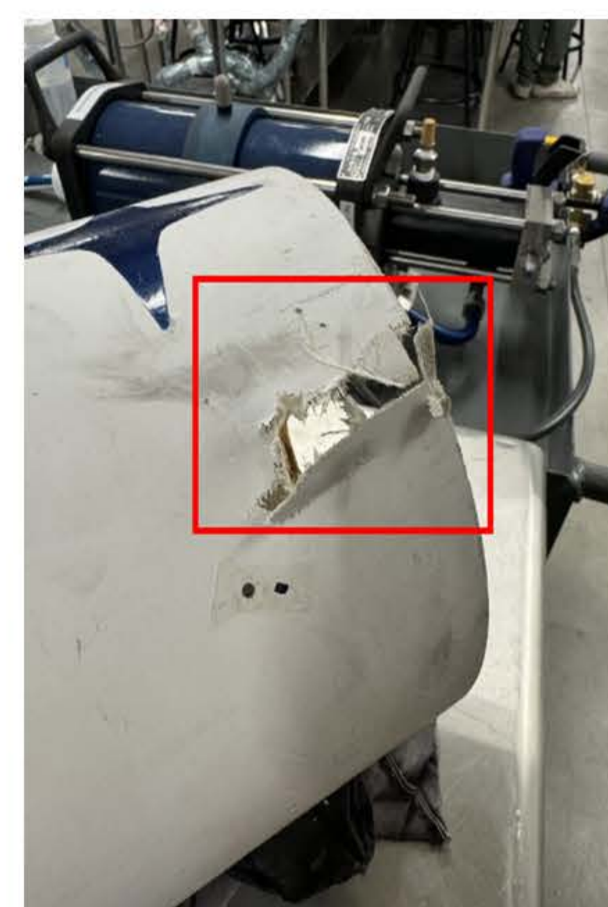
Figure 3 (left). Patriot rocket airframe experienced zippering potentially due to shock cord cutting through cardboard airframe.
