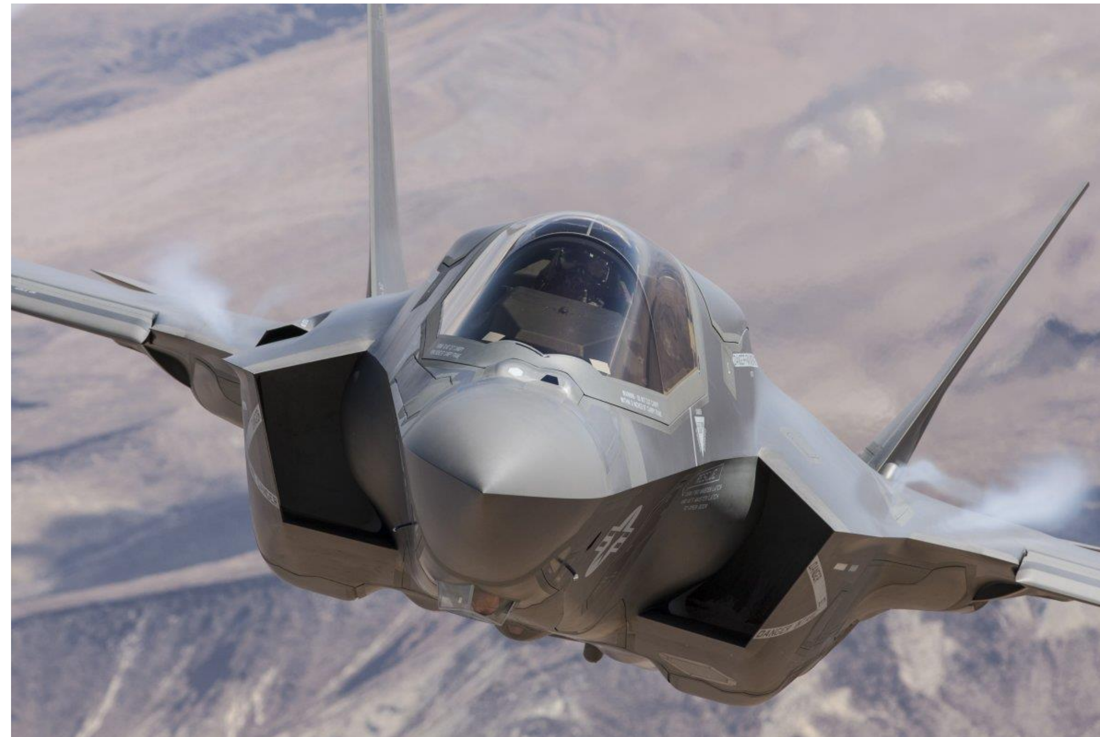
Diverterless Supersonic Inlets as Seen on the Lockheed Martin F-35 Multi-Role Stealth Fighter
