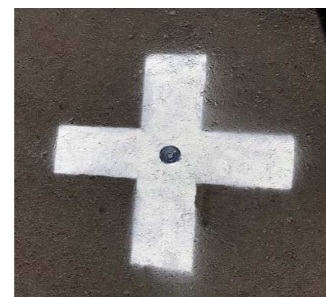
Figure 4. Aerial target for non-penetrable ground
