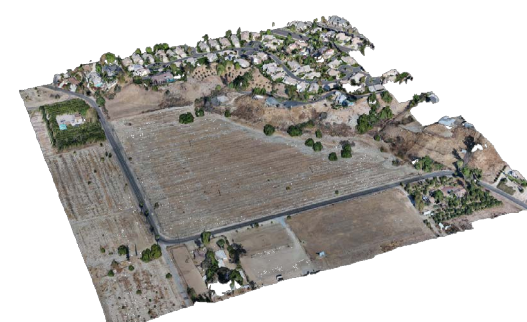
Figure 9. 3D surface model created from UAS photos using ContextCapture
