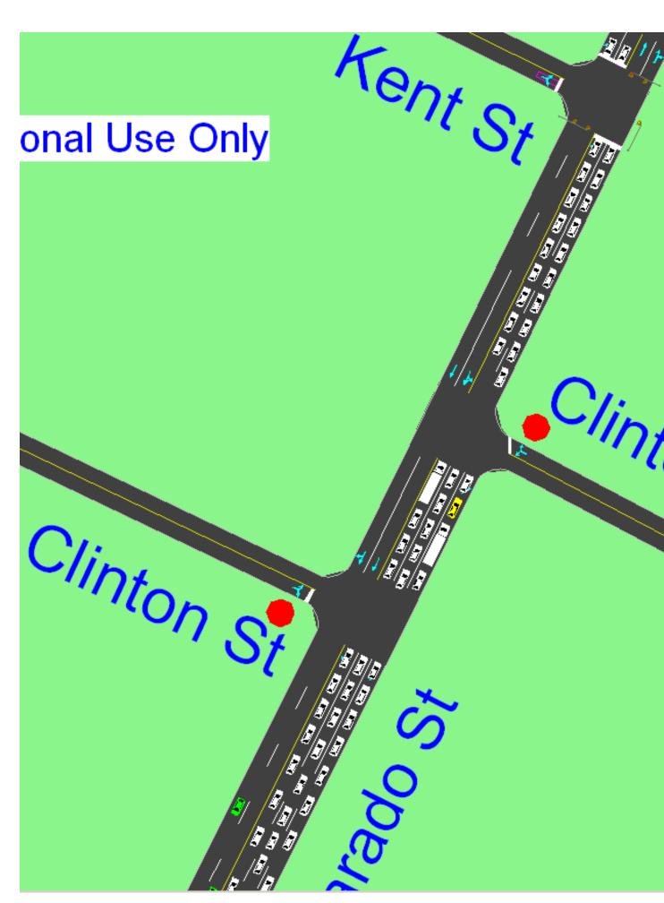
Placing a single pretimed signal will setback more than one intersection because it must designate time to a minor volume, decreasing other intersections' LOS.
