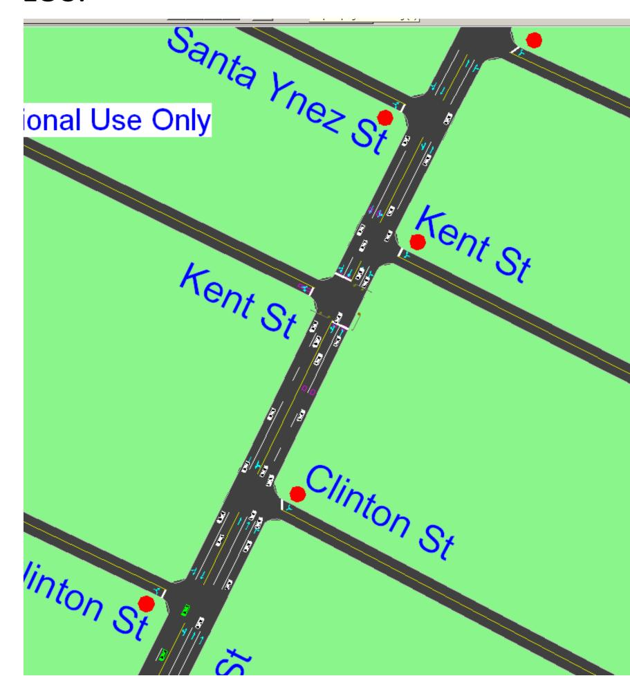
Establishing a semi-actuated signal will only designate time to a minor volume when it is present, which will allow free flow for the major volume most of the time.
