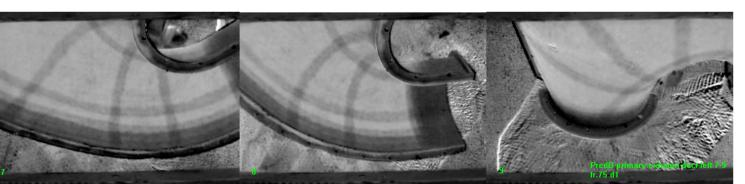
Pulse thermography of primary duct after 50 hours of testing(above).
