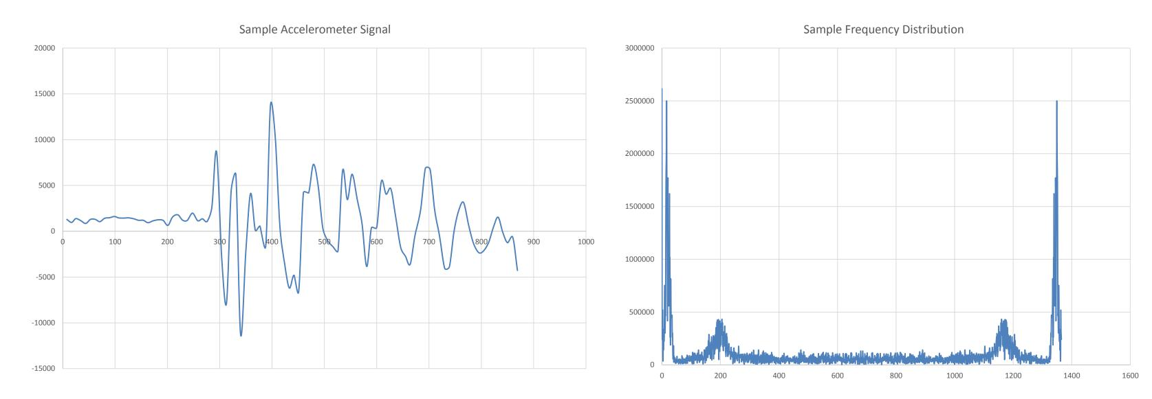
The above graphs illustrate the issue with the raw signal from the accelerometer. The graph on the left shows the signal, and the graph on the right shows the decomposition of the signal into its frequencies.
