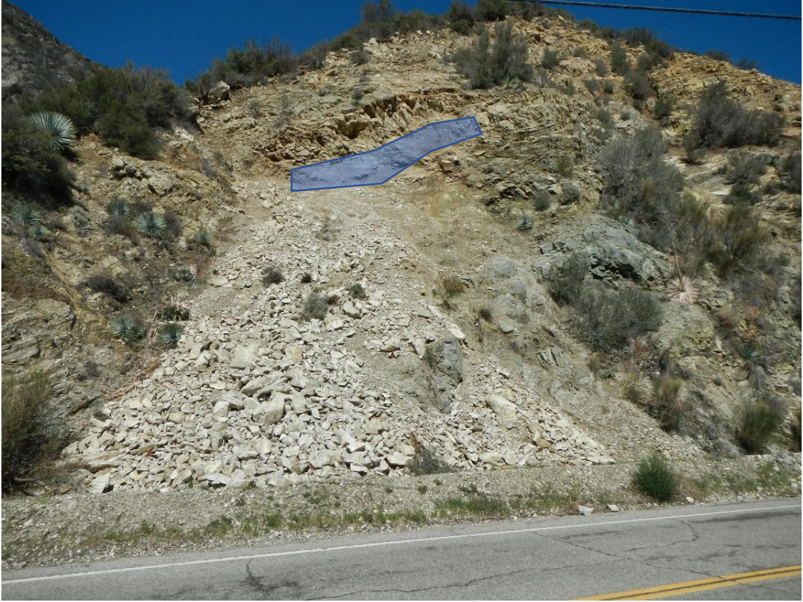
Figure 72: Image of the LS3 cone used to approximate the volume of material with slide surface in blue. Photo by Dr. Nourse February 11, 2019.
