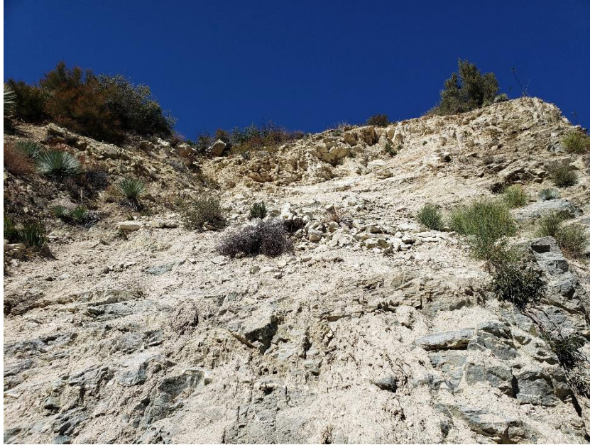
Figure 55: LS3 towards the top of the image with the breakaway point the steep surface on top. Seems to have a planar surface.
