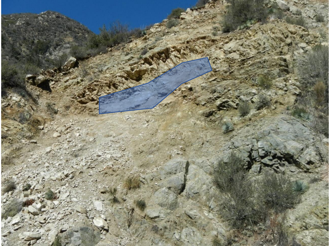
Figure 71: Photo of the failure surface of LS3 taken by Dr. Nourse on February 11, 2019. Suspected failure surface in blue. Some of the slide surface may still be buried so area could be larger. Scarp seen above the failure area.
