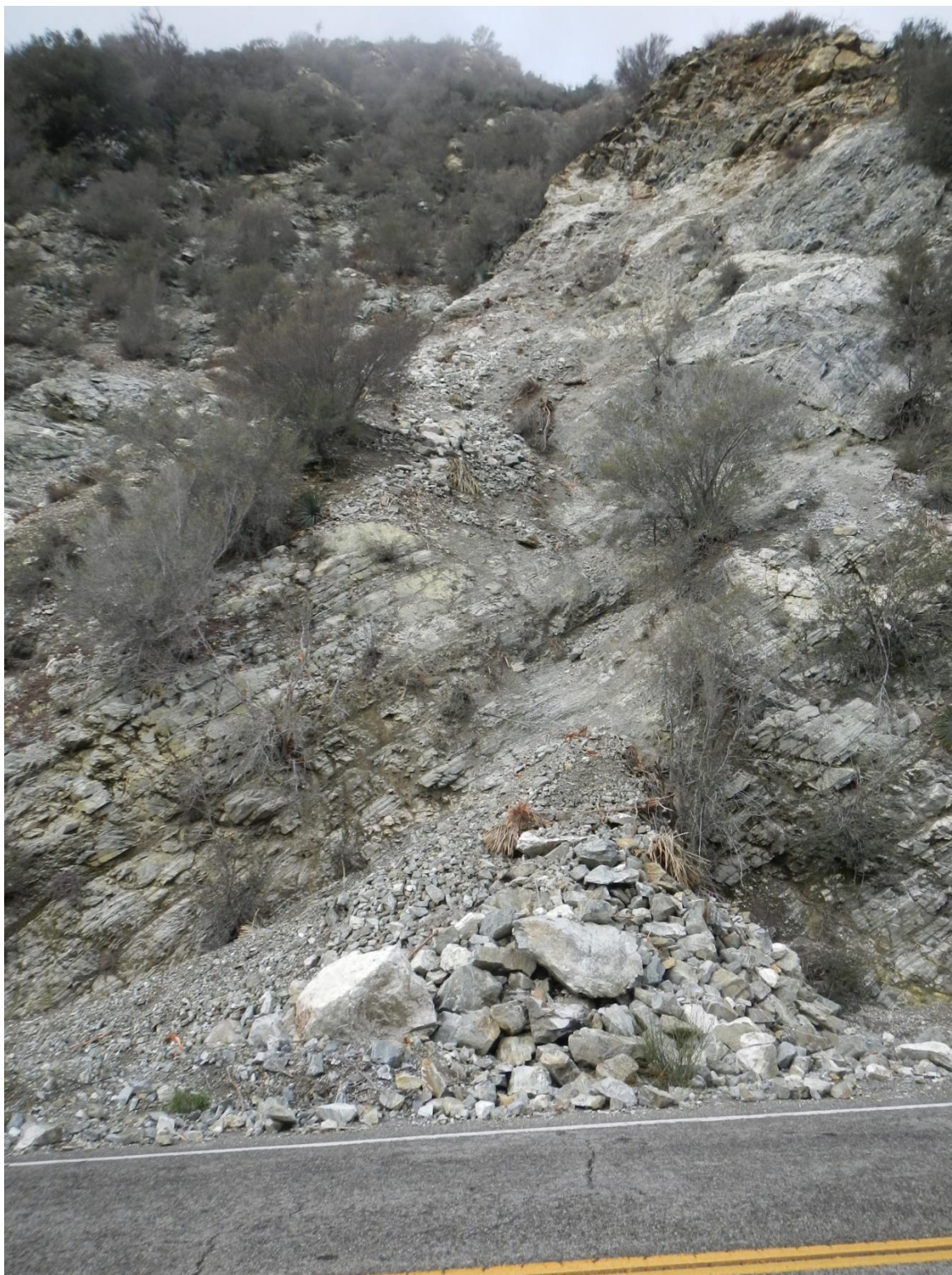
Figure 67: Photo of the cone of LS2 which was used to approximate dimensions by Laser Rangefinder after the debris were cleared. Photo taken by Dr. Nourse in 2017.
