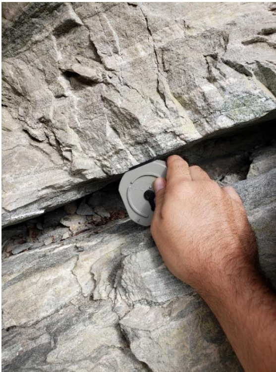
Figures 41 and 42: Figure 41 (left) shows the size of a fracture along the foliation plane in the felsic gneiss by the Sierra Powerhouse Access Road with Figure 42 (right) showing my mom taking notes from measurements.
