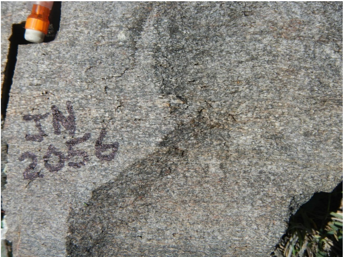
Figure 7. Close up of metasandstone geochronology sample JN 2056, collected northwest of Blue Ridge campground. In thin section, this sample contains garnet and displays replacement of chlorite with biotite.
