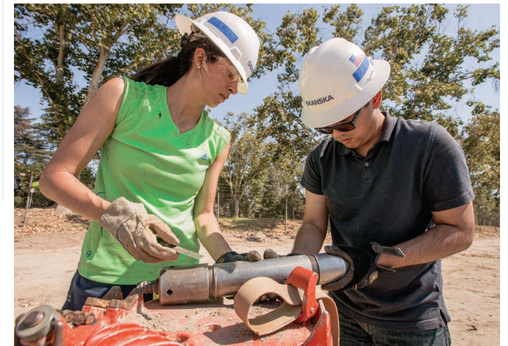
Civil engineering students collect soil samples for a geotechnical engineering lab class.
