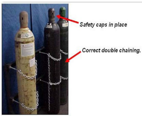
Cylinder stored and chained correctly
