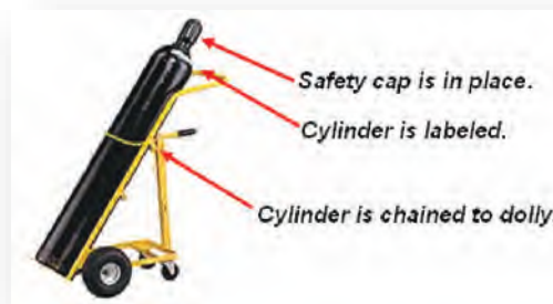
Correct cylinder transport
