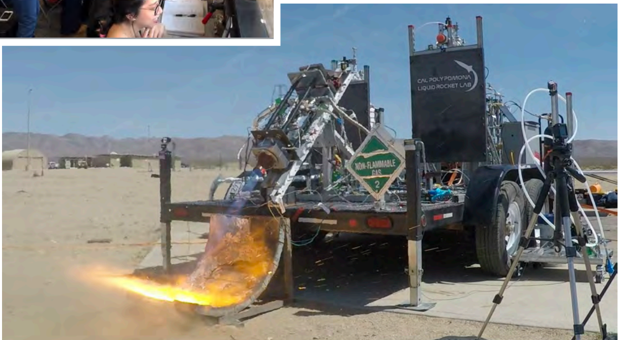
The team cheering after their first successful hot fire of their liquid rocket engine.
