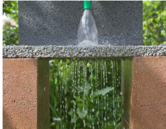
Figure 58: A demonstration of porous concrete pavers with water draining through.
