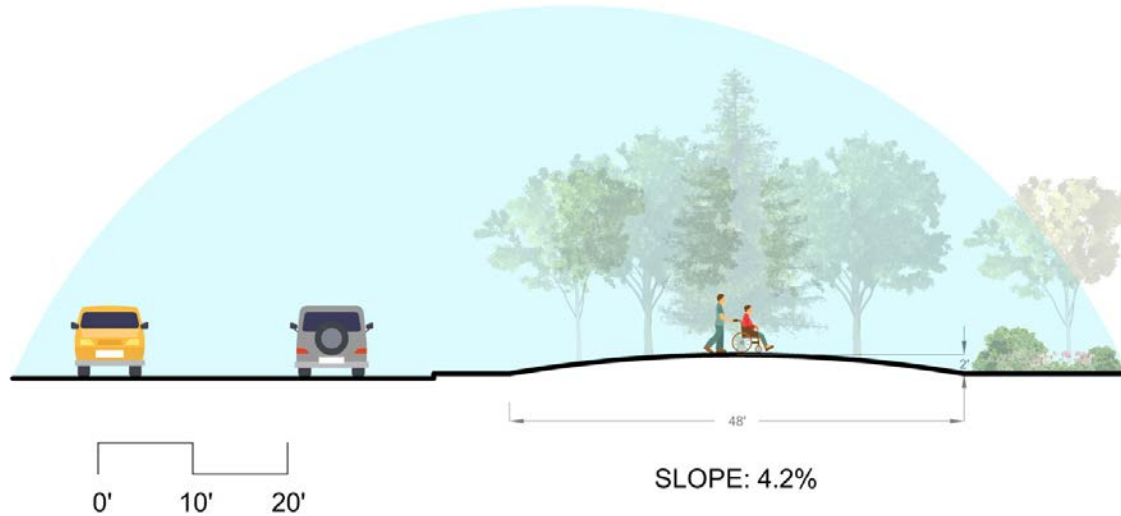
Figure 66: A section showing the water-retaining berm that surrounds the park. While entrance paths cross this berm, slopes have been calculated so that paths remain ADA-accessible.
