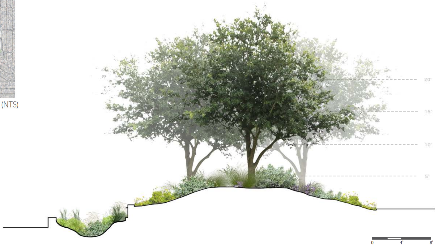
Figure 79: Typical Terraced Bioswale.
