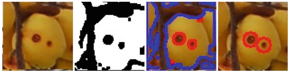
Fig. 10 Left to right Original apple image before segmentation; binary image after segmentation; external and internal contours; candidate regions of IFW damage
