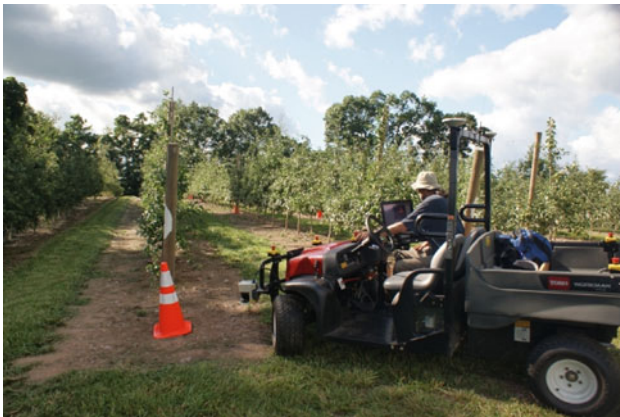
Fig. 7 The APM turns into a row of trees at the FREC. At that time the turn command was based on a predefined row width. Any deviation from that width could lead to overshoot or undershoot, causing the safety module to stop the vehicle
