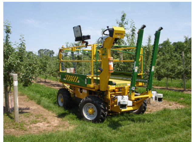
Fig. 9 The N. Blosi orchard agricultural platform converted into an automated orchard vehicle at the Pennsylvania State University Fruit Research and Extension Center
