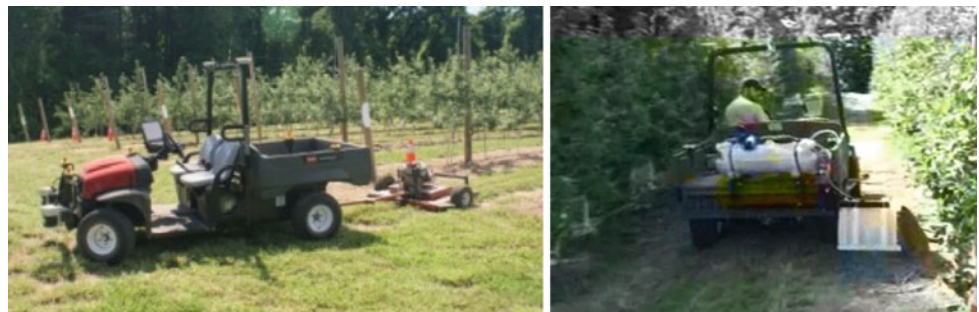
Fig. 8 Left The APM autonomously mows the grass in a block of trees. Right The APM autonomously sprays weeds with the NTech WeedSeeker
