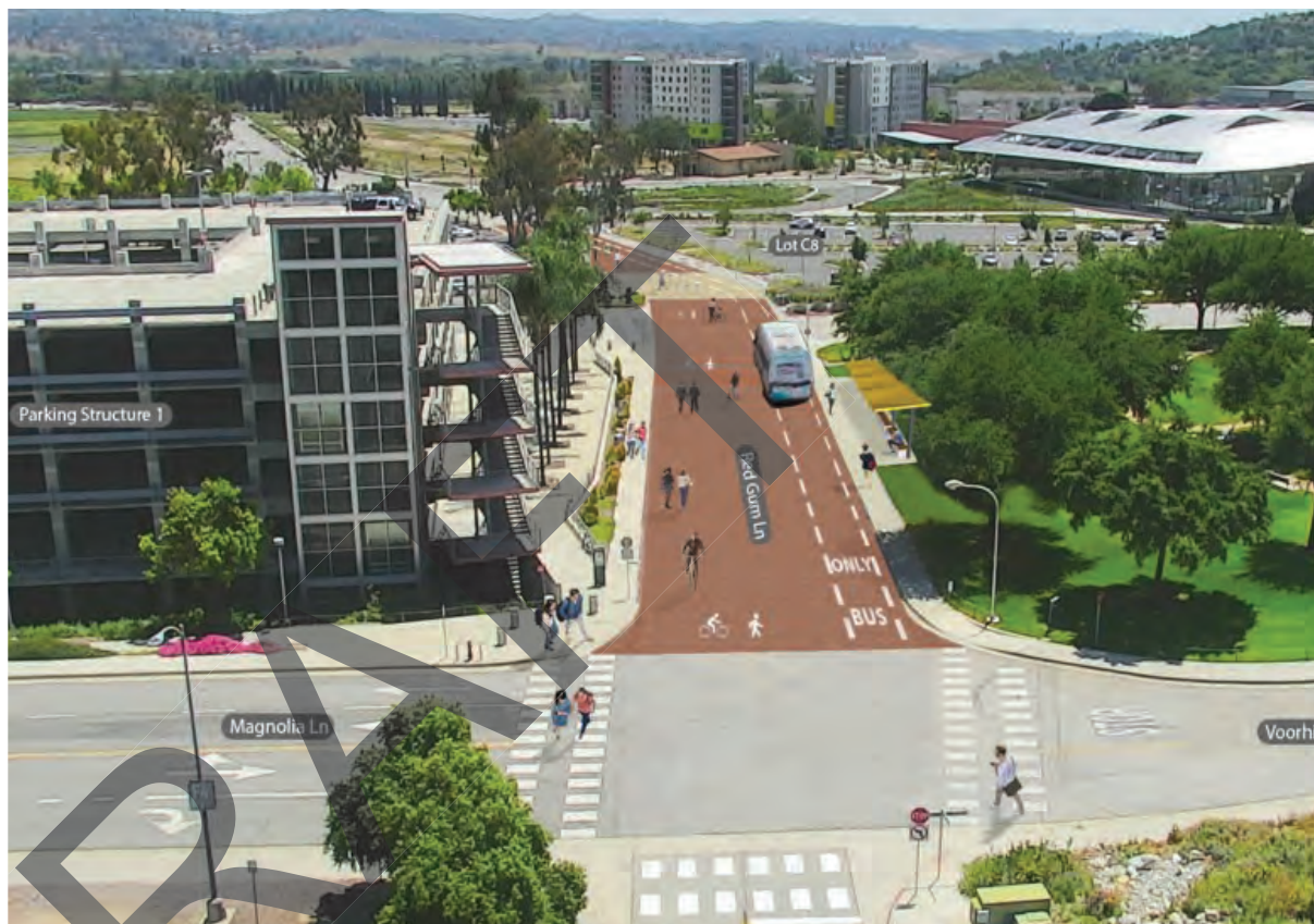
Red Gum Lane, which was partially closed to traffic, will become a multi-modal pedestrian mall including a lane for the campus loop shuttle, and new bus shelter with PV solar shade, continuing the conversion of former streets to pedestrian malls.
