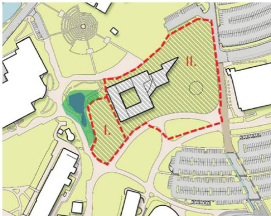
Bldg 98 site restoration: Phase I is the demolition footprint that was restored for student use (completed). Phase II includes the original street and drop-off circle and loading/service areas.
