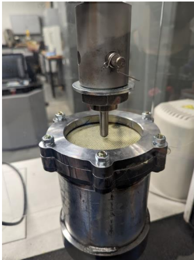
Figure 10: Hemispherical Impactor set up.
