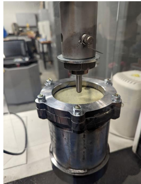
Figure 4: Set up of the quasi-static test fixture using the hemispherical impactor.
