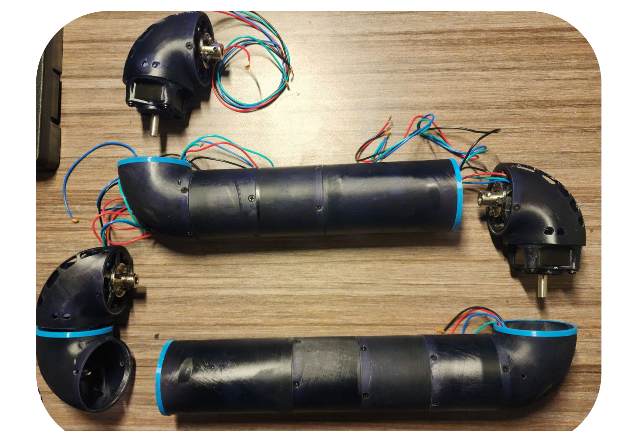
Figure 10: The components pre-assembly, wires soldered and ran through the tubes
