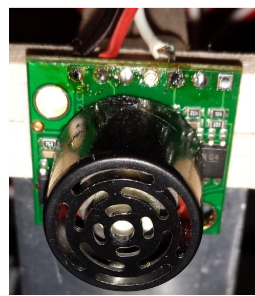
Figure 2. Maxbotix LV-EZ0 Ultrasonic sensor
