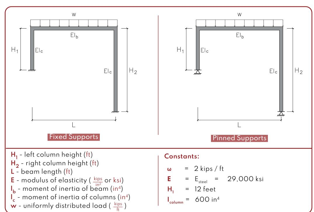
Aside from the variations in the support conditions, recommendations of hinges are also based on a set of parametric studies involving variations in column heights, beam span and moments of inertia
