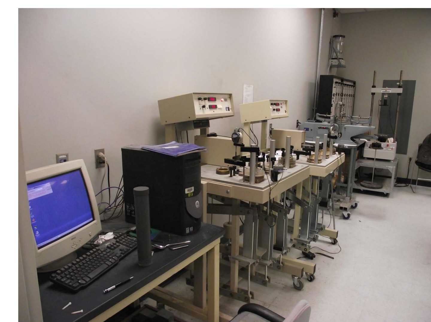
Figure 3. Direct Shear machine setup used to test mixture's strength.
