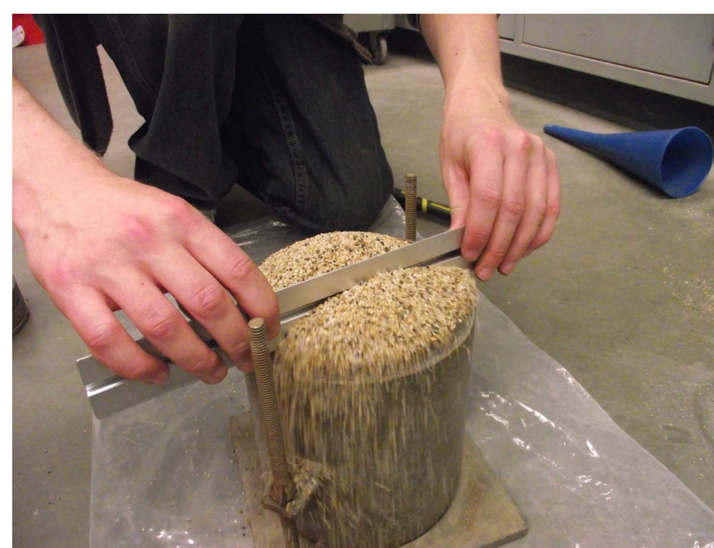
Figure 2. ASTM mold used to test unit weights.
