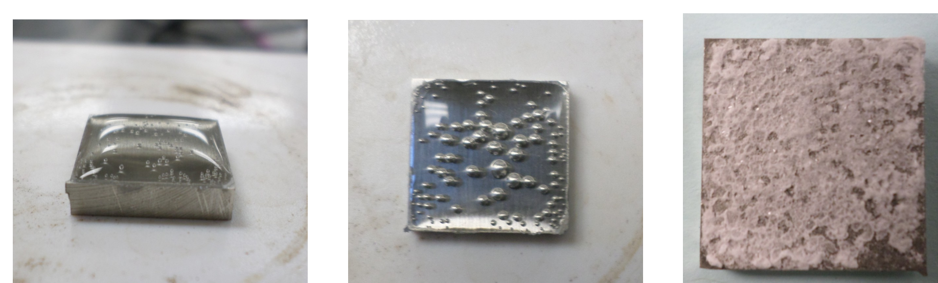
Figure 4-1: (a) Salt solution applied (b) Water begins to evaporate (c) Resulting tenacious salt film
