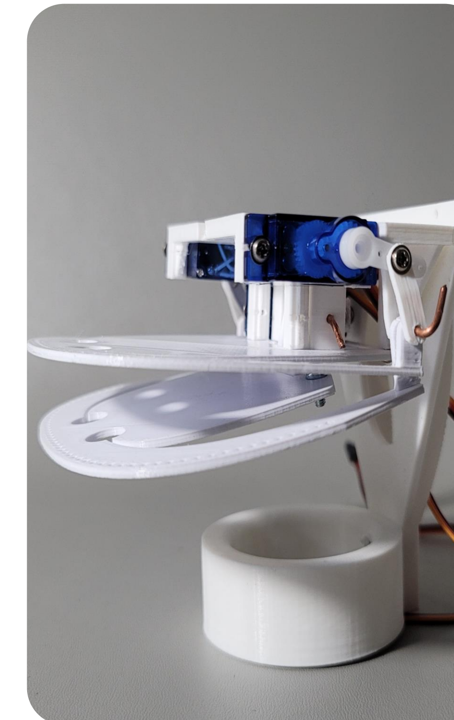
Figure 3. This image shows the circular base, back neck plate and both jaws for the unit. Copper wire is used at crucial hinges/levers that need to rotate to allow for the mouth to function.
