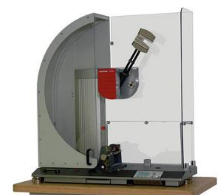
Pendulum test can be used to simulate the impact
