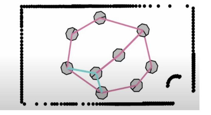
Real-Time Appearance-Based Mapping (RTAB-Map) is a variation of GraphSLAM which can be split into two processes, the front-end and back-end as shown in the diagram below.
