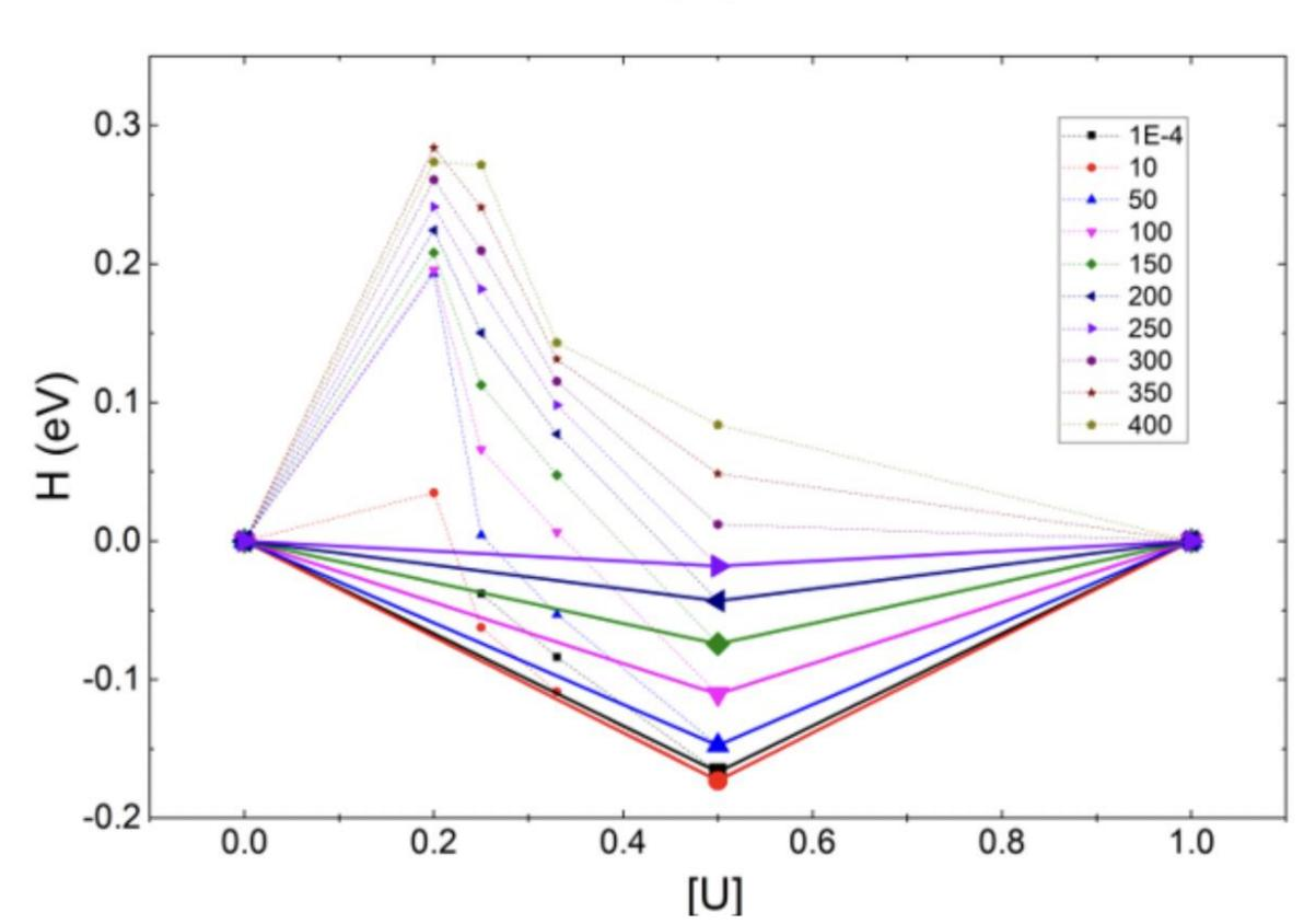
This is an example of a convex hull, with the enthalpy of formation on the y-axis and the Uranium content on the x-axis (Botana, McGarvey, Gilbert). The convex hull plots the enthalpy of formation of a compound as a function of Uranium concentration and pressure. Each point corresponds to a different pressure. It allows us to deduce the spontaneity of compounds, if they will form or not, and if they are stable.
