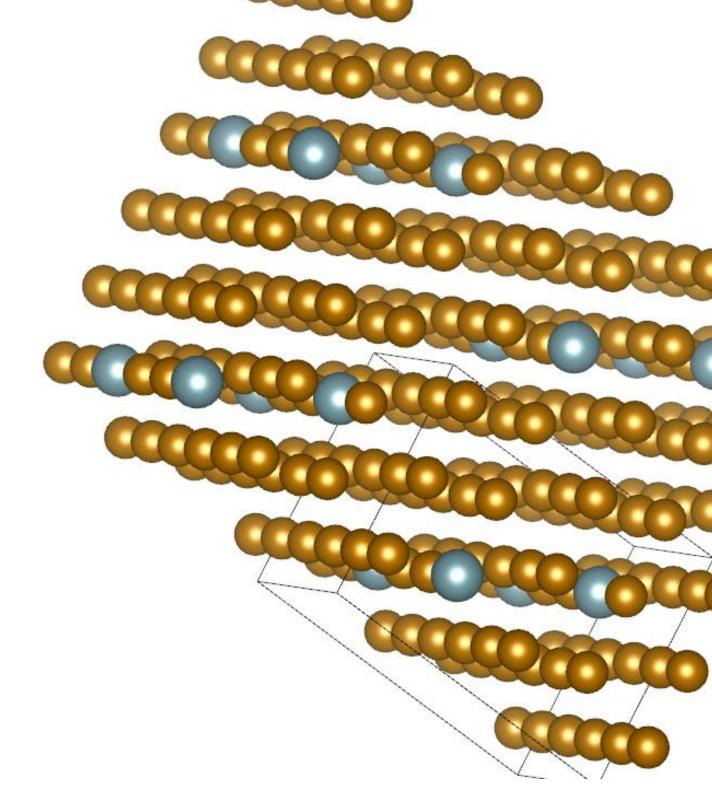
This is a visualization of an Iron compound with Uranium impurities. The locations of the atoms are stored, and we input this file (visualization through VESTA) into VASP to do our calculations. Using the locations of the atoms and a pseudopotential, VASP calculates the entropy of this sample. Different geometries of atoms yield different enthalpies.
