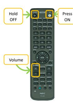
The projector can be turned **ON** by pressing the ON button on the included remote. To turn the projector **OFF**, press and hold the Standby button until you receive a prompt and confirm.
