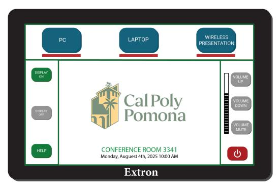
Across the top you will find the different inputs based on the device you want to display on the projector.
