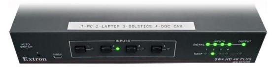
**Laptop Input:** This input source utilizes a loose HDMI cable around the lectern. If your computer does not support HDMI, a set of adapters for USB-C, DisplayPort, and Mini DisplayPort can be found within the lectern. If you cannot locate it, contact classroom
