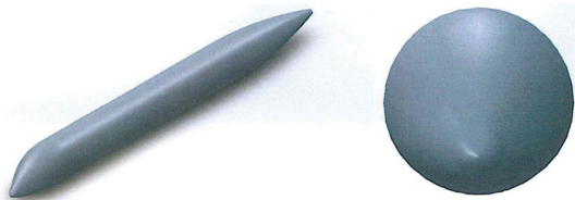
Figure 3: 3-D CAD Model of Un-dimpled 787 Fuselage
