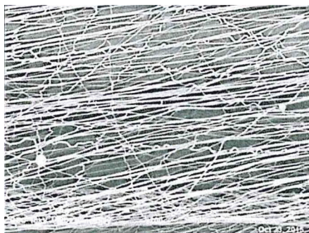
Figure 4: Sodium-Cobalt Oxide Nanofiber Distribution
