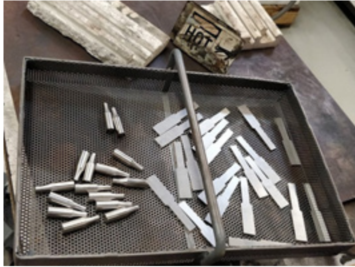
Figure 5 – Machined samples prior to being placed in the furnace
