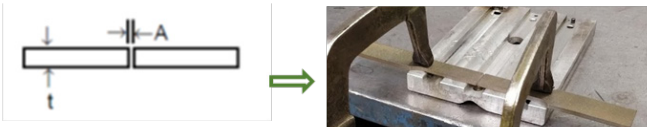
Figure 8 – Weld preparation and layout of tension samples
