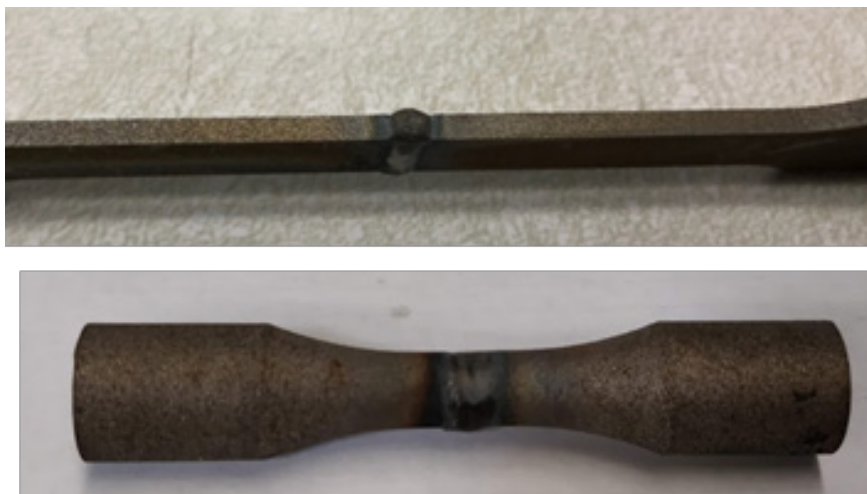
Figure 10 – Actual samples after welding
