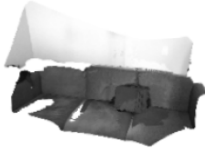
Figure 3. Point clouds are aligned after Fast Global Registration and Colored ICP registration.
