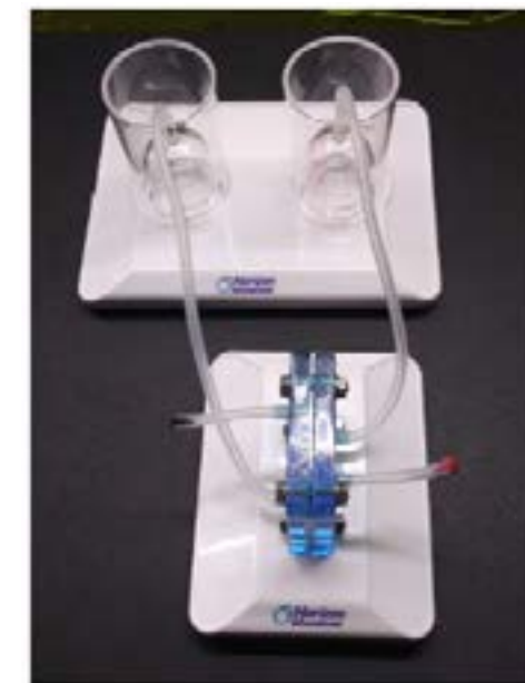
Figure 2. Set up of fuel cell kit before electrolysis began.
