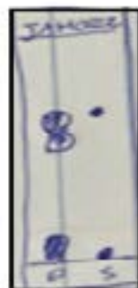
Figure 2. Represents a TLC plate of the starting material labeled "S" (3-hydroxyphenyl acetic acid) and the product labeled "P" (methyl 3-hydroxyphenyl acetate). The overlapping in the dots showed there was impurities within the sample there no yield was able to be obtained.
