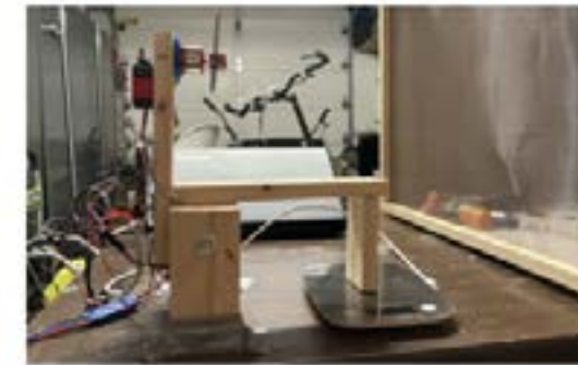
Figure 17: Thrust Test Bench Mechanism
