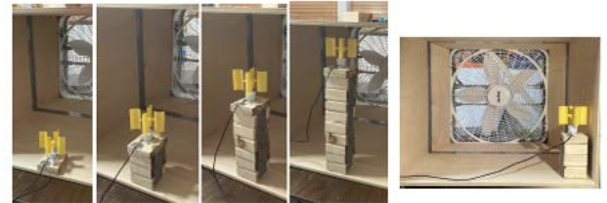
Figure 11: Anemometer at Various Positions in Wind Tunnel
