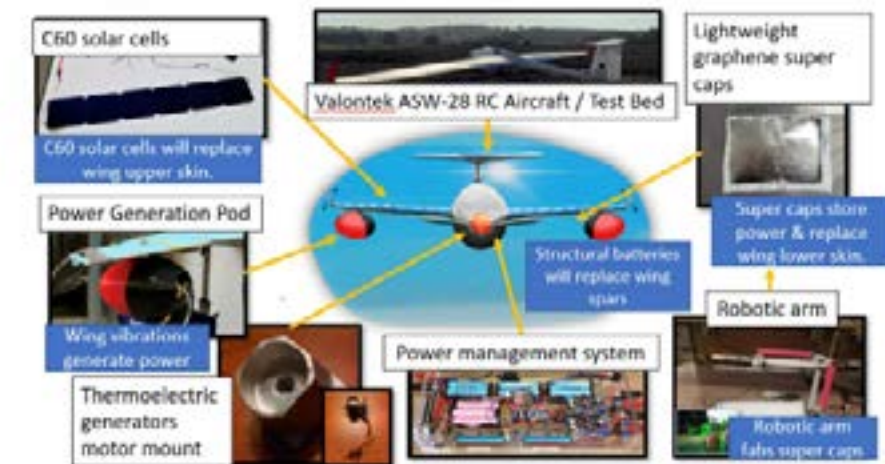
Figure 1.1 Replace aircraft structure with power storage and power structures to reduce weight and increase flight endurance
