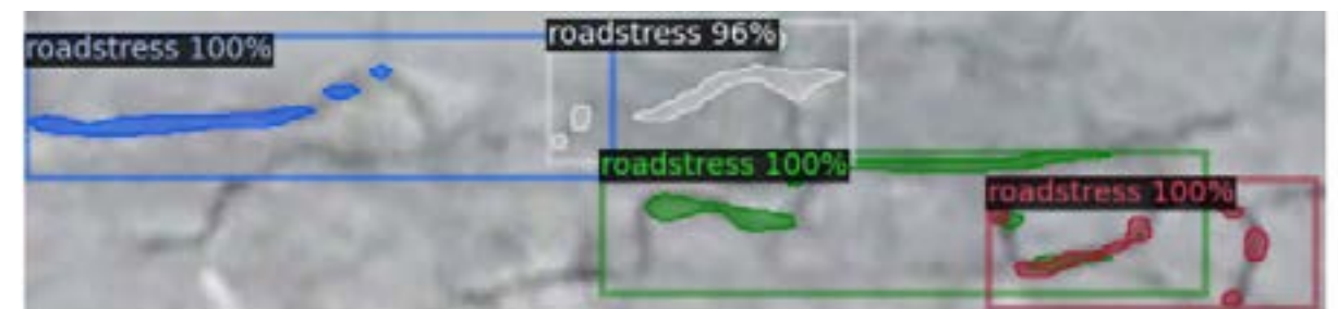
Figure 9: Example of false-negative recognition of road stress by the algorithm.
