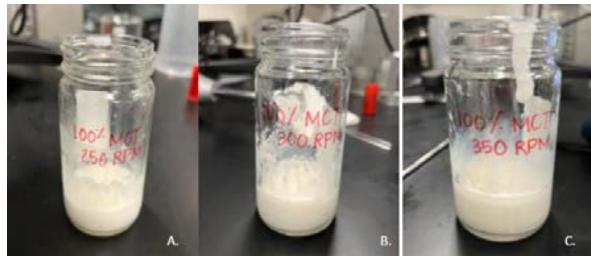
Figure 2. Water in oil Emulsions created with a 100% water aqueous phase
