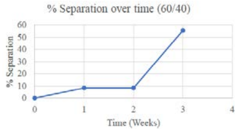
Figure 6. Separation over time graph for an emulsion prepared with a 60 vol% water and 40 vol % ethanol aqueous phase
