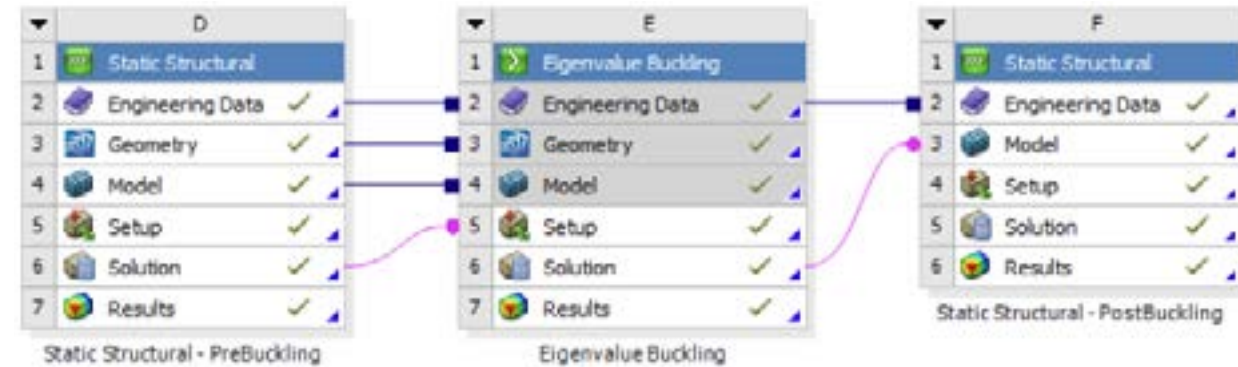
Figure 4 - ANSYS modules for static buckling analysis.
