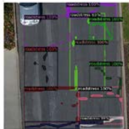
Figure 6: Example of successful recognition of road stress by the algorithm from a drone image.
