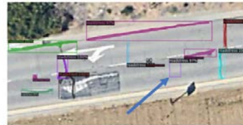
Figure 8: Example of false-positive recognition of road stress by the algorithm.
