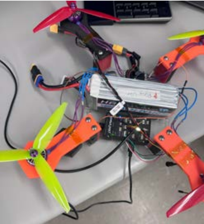
Fig. 8: Updated Top-Half of UHV Linked to Raspberry Pi 4
