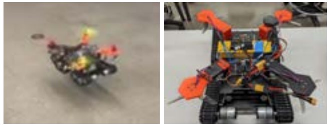
(a) Unmanned Hybrid Vehicle Flying in Flight Test (b) Older Version of Current UHV Prototype
