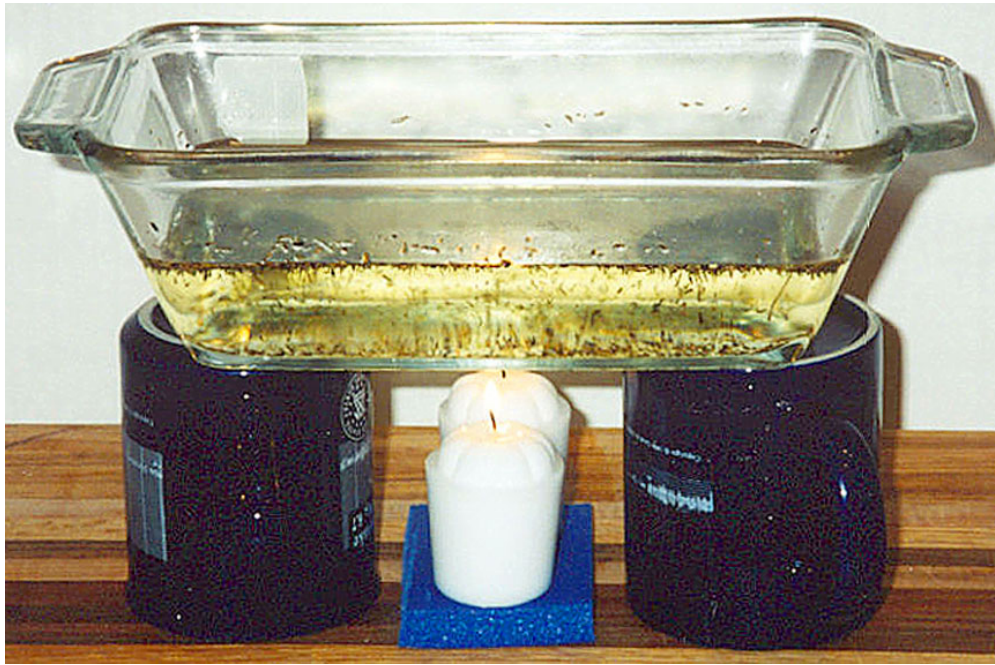
Figure 2. Alternate setup using two candles instead of the Sterno for heat.
