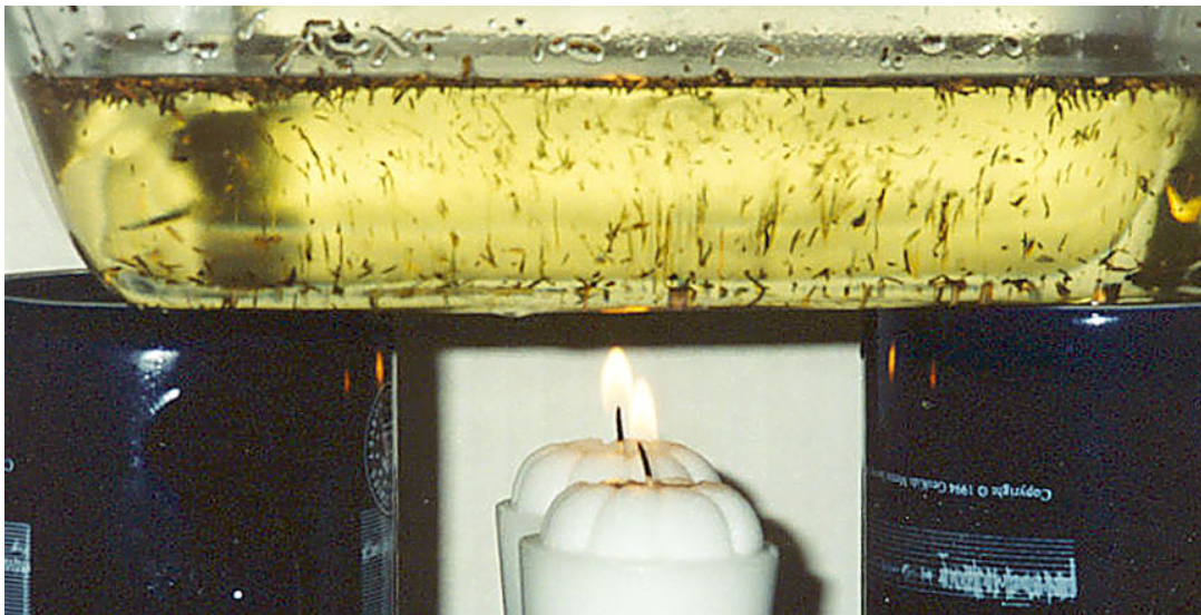
Figure 3. Close-up photo (side view) of the oil and thyme in the glass dish. Heat from the candles causes the oil and thyme to rise in the middle of the dish (above the candle flames), flow horizontally (away from the center) near the surface of the oil, sink near the cooler edges of the glass dish, and flow horizontally toward the center along the bottom of the dish, thus completing the convection cells.
