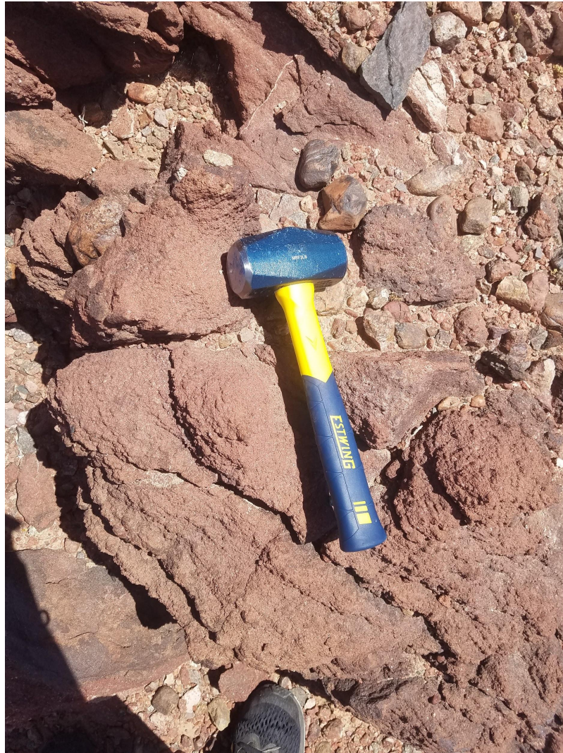
Appendix D.41. West - matrix finer grain compared to conglomerates above. Indication of white calcite layer - looks to be a darker red sandstone layer - cemented. Hammer for scale
