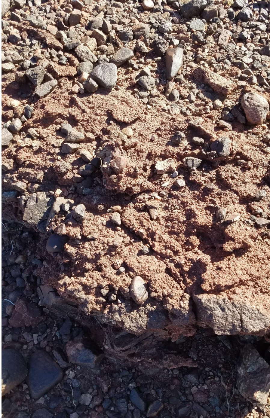
Appendix D.63. East - area of first sample taken after ignimbrite - shows variety in grain sizes - rounded to sub rounded grains
