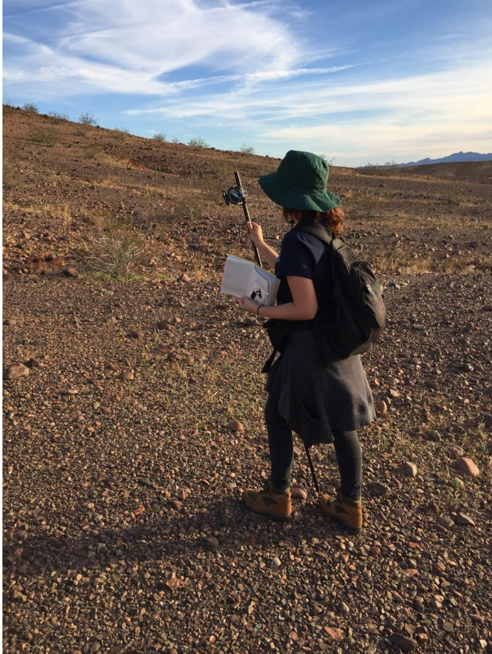
Appendix D.28. TT canyon - Construction of western stratigraphic column (A-A') using Jacob staff and brunton compass.
