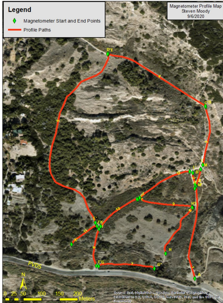
Figure 3.12. Magnetic survey profiles are numerically labeled and their starting and ending locations are marked alphabetically. PVDS marks Palos Verdes Drive South.
