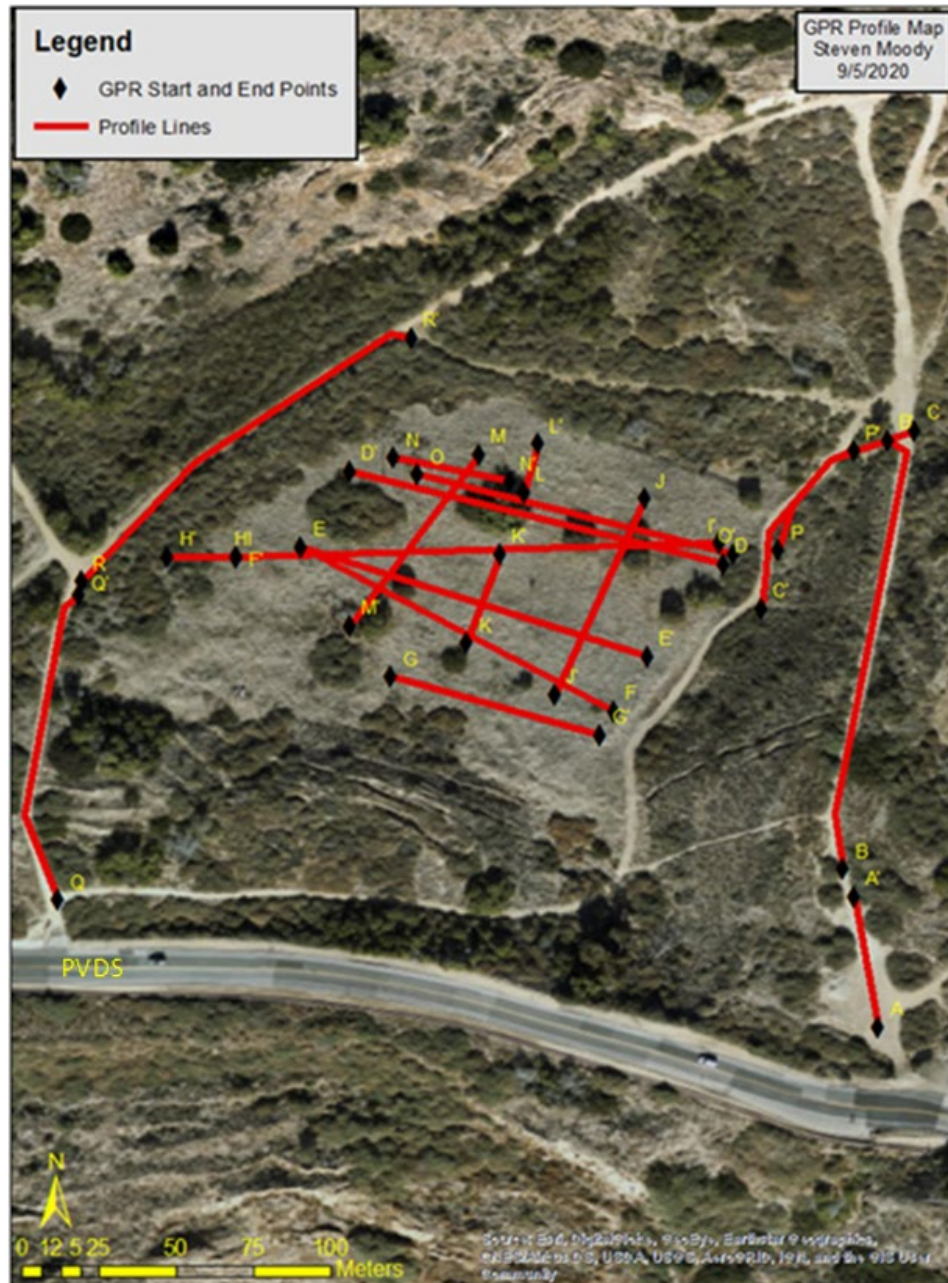
Figure 3.9. Map generated in Esri's ArcMap 10.6.1 software. GPR profiles and paths are displayed as well as their respective start and end points. Profiles were recorded with alphabetical designation. PVDS marks Palos Verdes Drive South.
