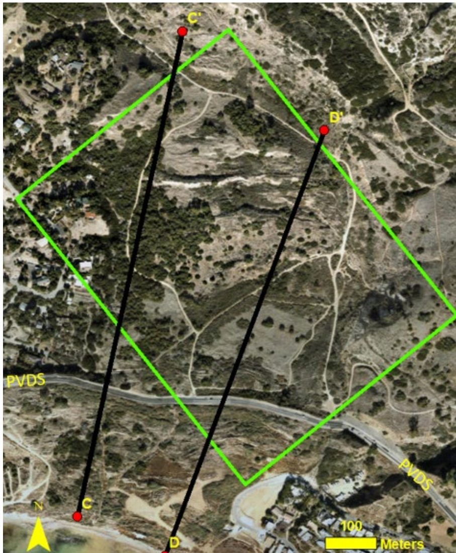
Figure 1.11. The field area is displayed with two of the four lines Ehlig used to create his cross sections. Sections A-A' and B-B' fall outside of the surveyed area. The rough extent of the field area is enclosed in the green rectangle. PVDS is Palos Verdes Drive South.
