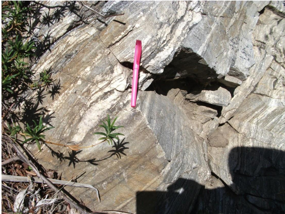
Figure 23. Photo of the felsic gneiss jointing and foliation orientations, in-place.
