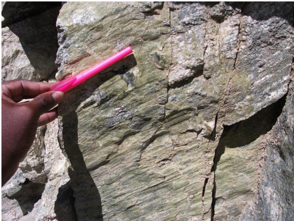
Figure 33. Photo of an epidote surface, showing the direction of the rake.
