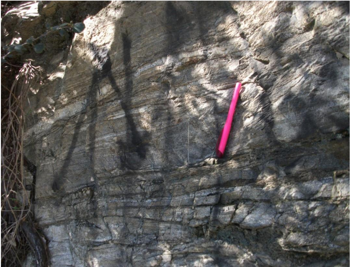
Figure 19. Photo of the Felsic Gneiss in-place, showing typical metamorphic foliation.
