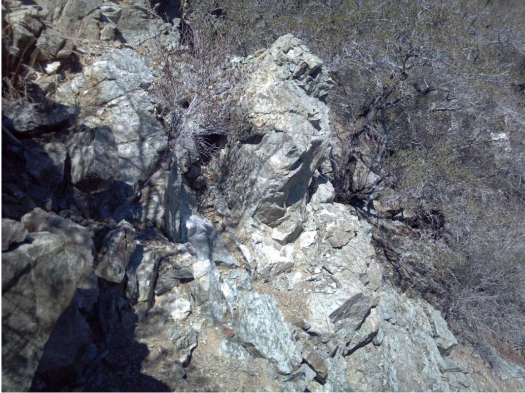
Figure 18. Photo of the fractured and weathered quartz diorite on the Hog Back Slide scar
