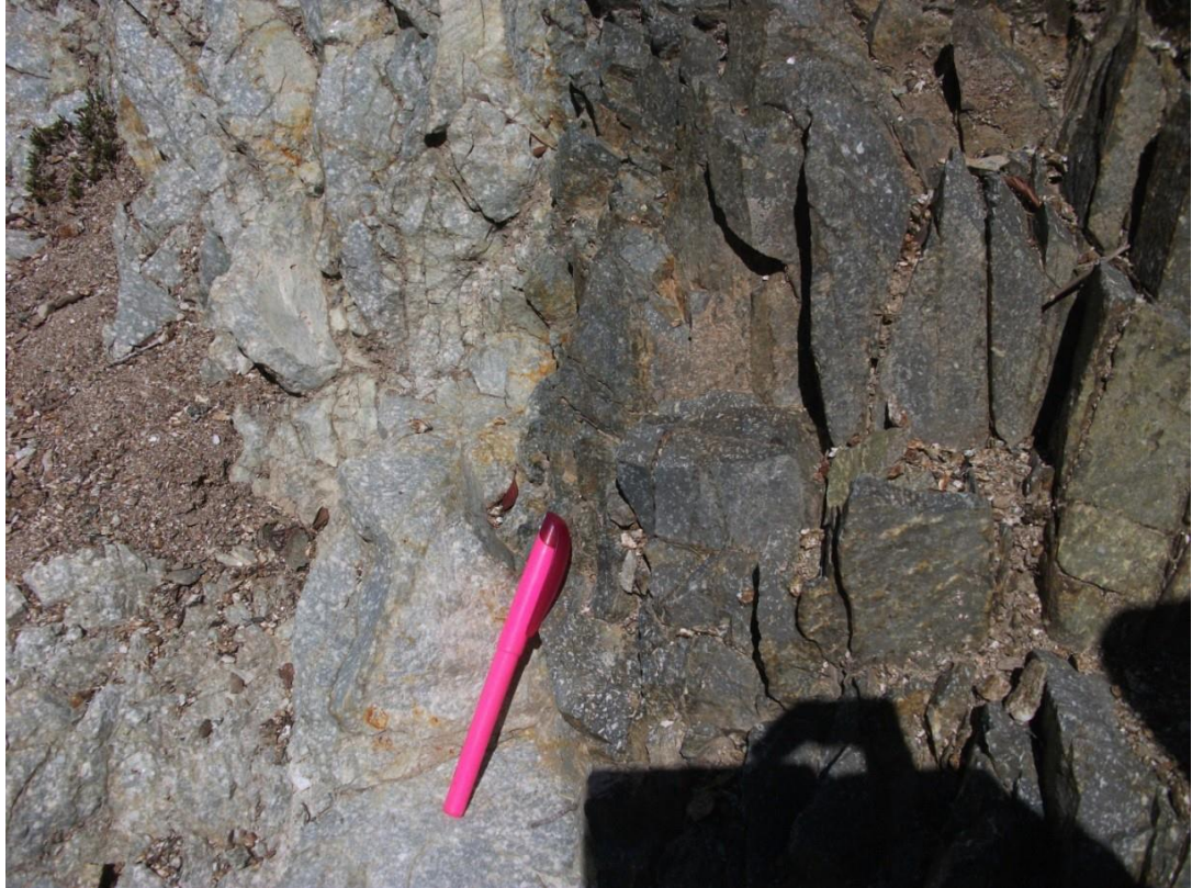
Figure 37. Photo of mafic dike within felsic gneiss.
