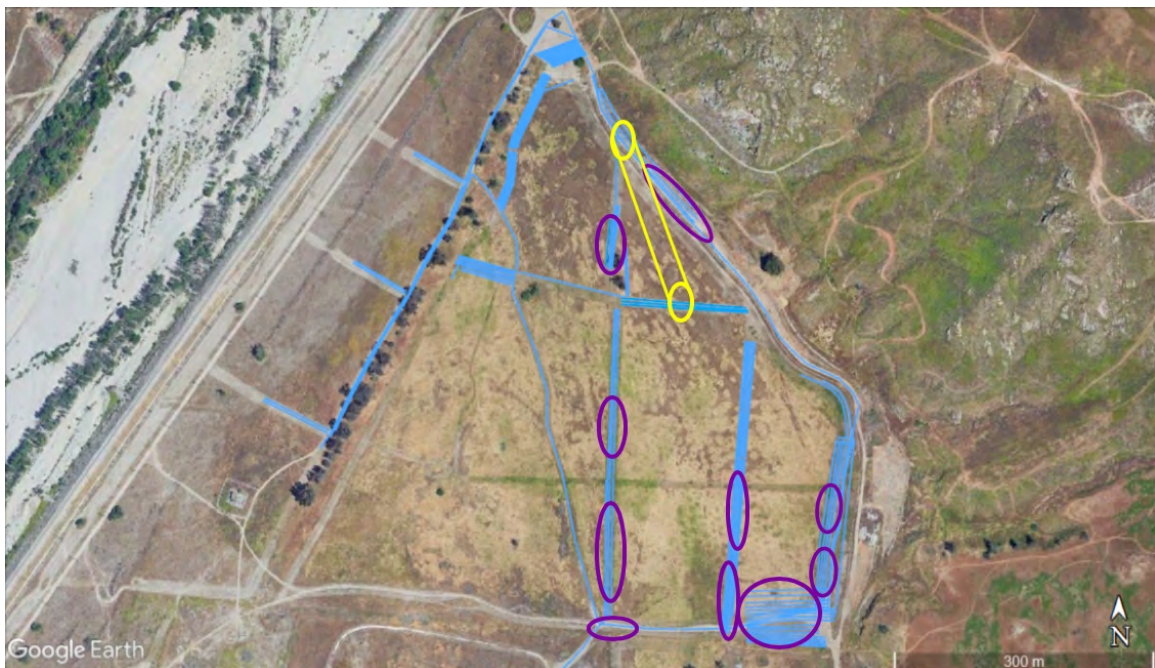
Figure 48: Map of all major GPR anomalies. The labels point out those shown in this section. Features are circled in purple and labeled by their Figure number. Yellow circles with connecting lines drawn as probable path of irrigation canal, based on GPR data at the two circled locations, which show a similar sized and structured canal, decreasing in width from 13 to 5 meters as its distance from the SAR increases. We hypothesize that in the 13-meter measurement of the canal, we had run more diagonal, instead of perpendicular, to the canal.
