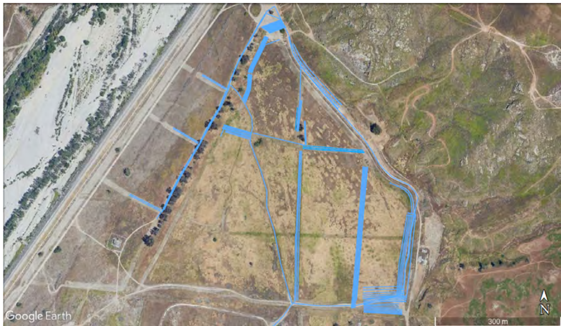
Figure 29: Overview of all GPR lines collected at Pellissier Ranch represented by blue lines (Google Earth Pro, 2018).
