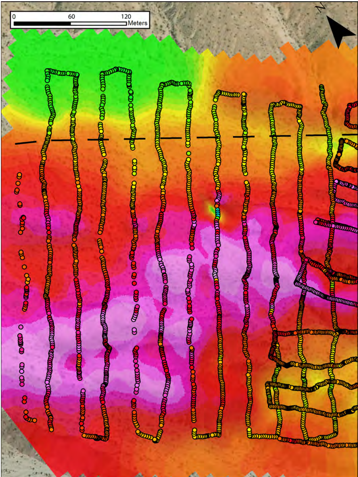
Figure 28: Interpolated total field intensity map of Bonanza Springs with collected data points overlain. Map shows a portion of the measurements across the north-west trending fault zone to demonstrate collected data values match contoured gridded values. Same color scale as Figure 27.
