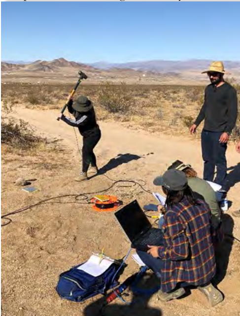
As before, the seismic source is a student-powered sledge hammer.
