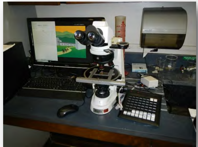
Our Pelcon point-counting system, with one of the new Nikon microscopes.
