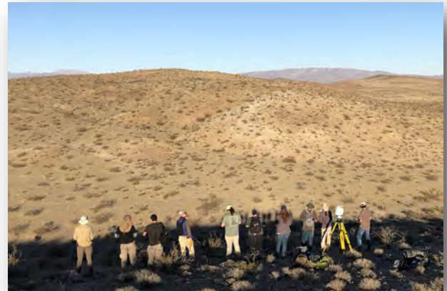
LiDAR—GSC 5030L students take notes while our new terrestrial laser scanner measures the Ridgecrest earthquake surface rupture below.
