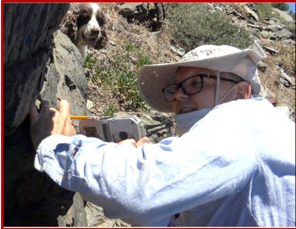
Measuring the trend of a fold hinge on Blue Ridge.
