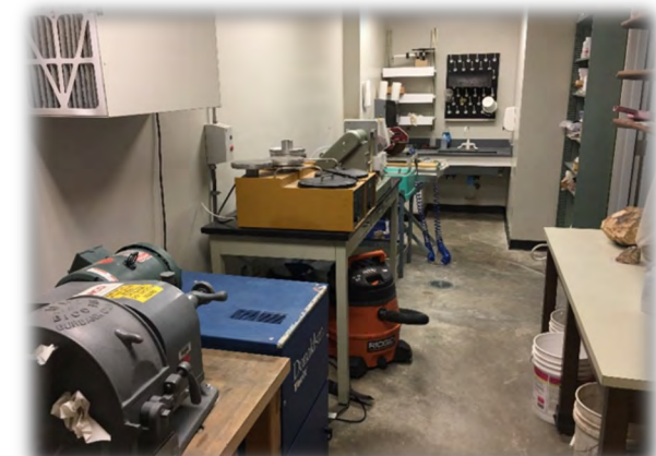
Our newly reorganized rock prep room (4-A-639B). View from the rock crushing area shows Bico pulverizer and dust collection system on the left foreground with polishing equipment, thin section machine and rock saws farther back.
