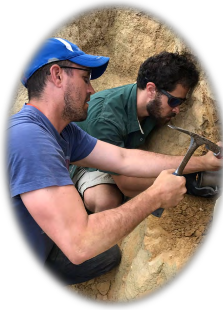
Noah Zohbe and Caleb Miller extracting OSL sampling tube from uplifted Pleistocene marine terrace cover beds, Riversdale, New Zealand.
