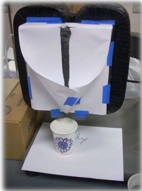
The first step in vertical Frantzing is to remove the iron filings produced by the rock pulverizer.
