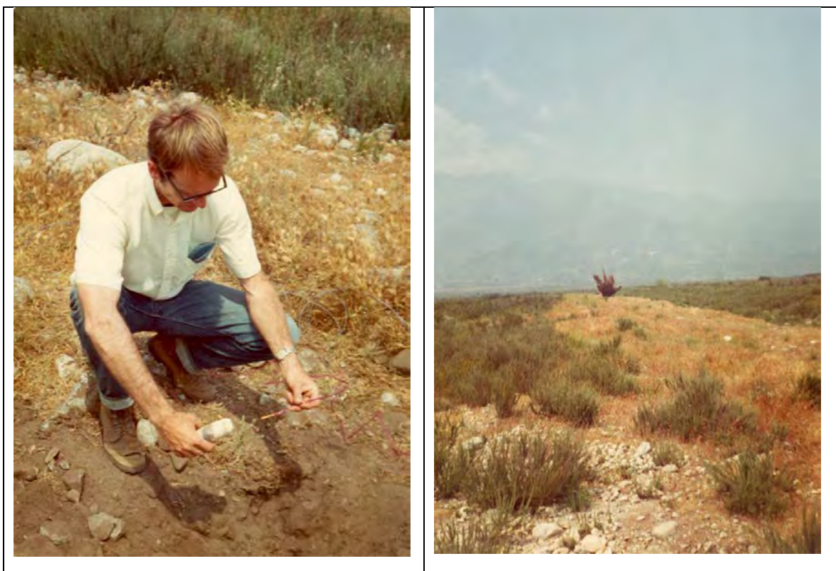
Left - Prof. Don Tarman inserting blasting cap into 12 ounce can of ANFO at Chaffey College demonstration. Right image shows actual detonation from about a quarter-mile distance.
