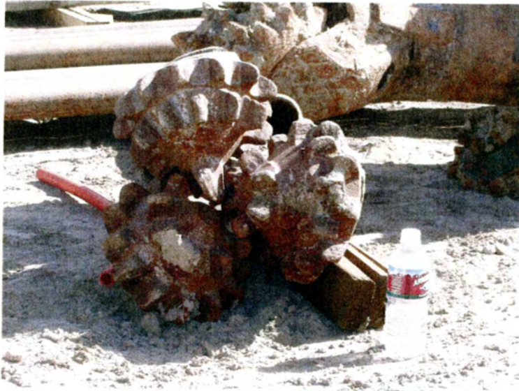
17½-inch diameter tri-cone button bit
