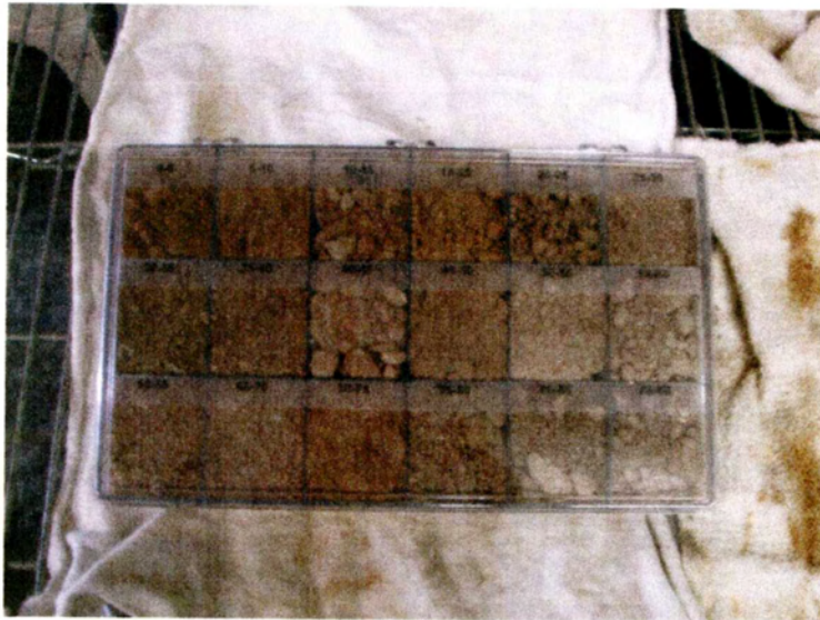
Chip trays showing continuous borehole section
