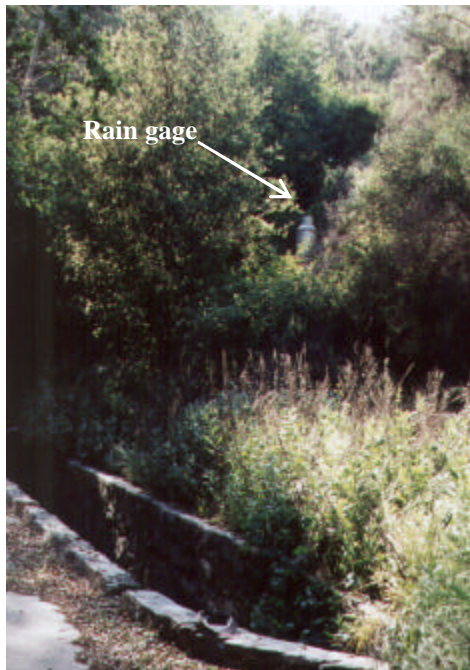
Figure 4 - The rain gage at Bell Dams is hidden behind the brush. The initial location was probably not heavily forested. Vegetation overgrowth has engulfed the rain gage and may have an effect on more recent precipitation values.
