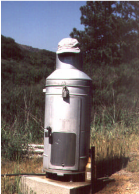
Figure 2 - Rain gage at Tanbark Flats. All monitoring equipment is housed in an alloy shell. Data recording instruments are located in a chamber at the base of the rain gage. (Baseball cap for scale)
