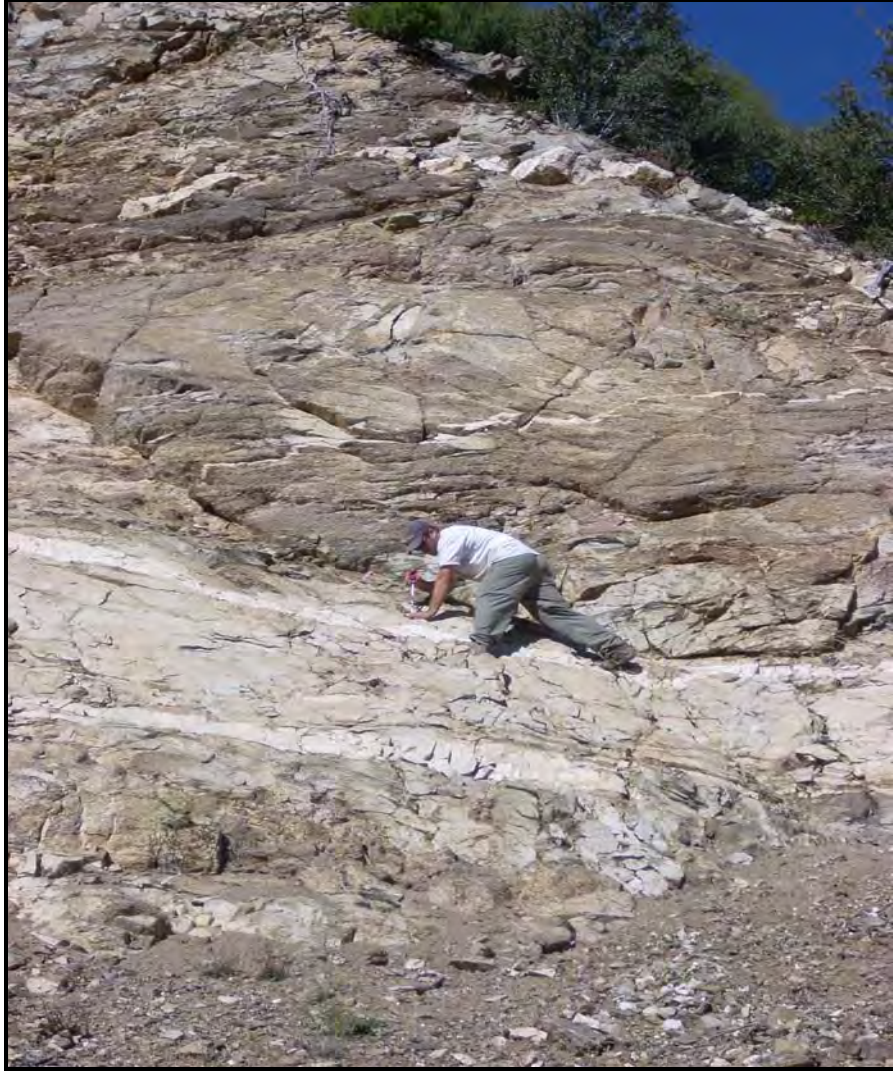
Figure 5. Using the surveying prism to mark the daylighting fracture which is oriented sub-parallel to the lower slide surface.
