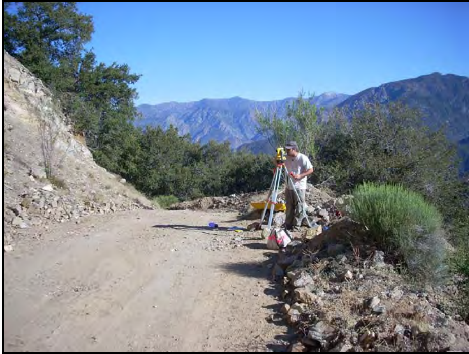
Figure 4. Surveying using the Trimble Total Station on the fire access road directly beneath the landslide scarp.
