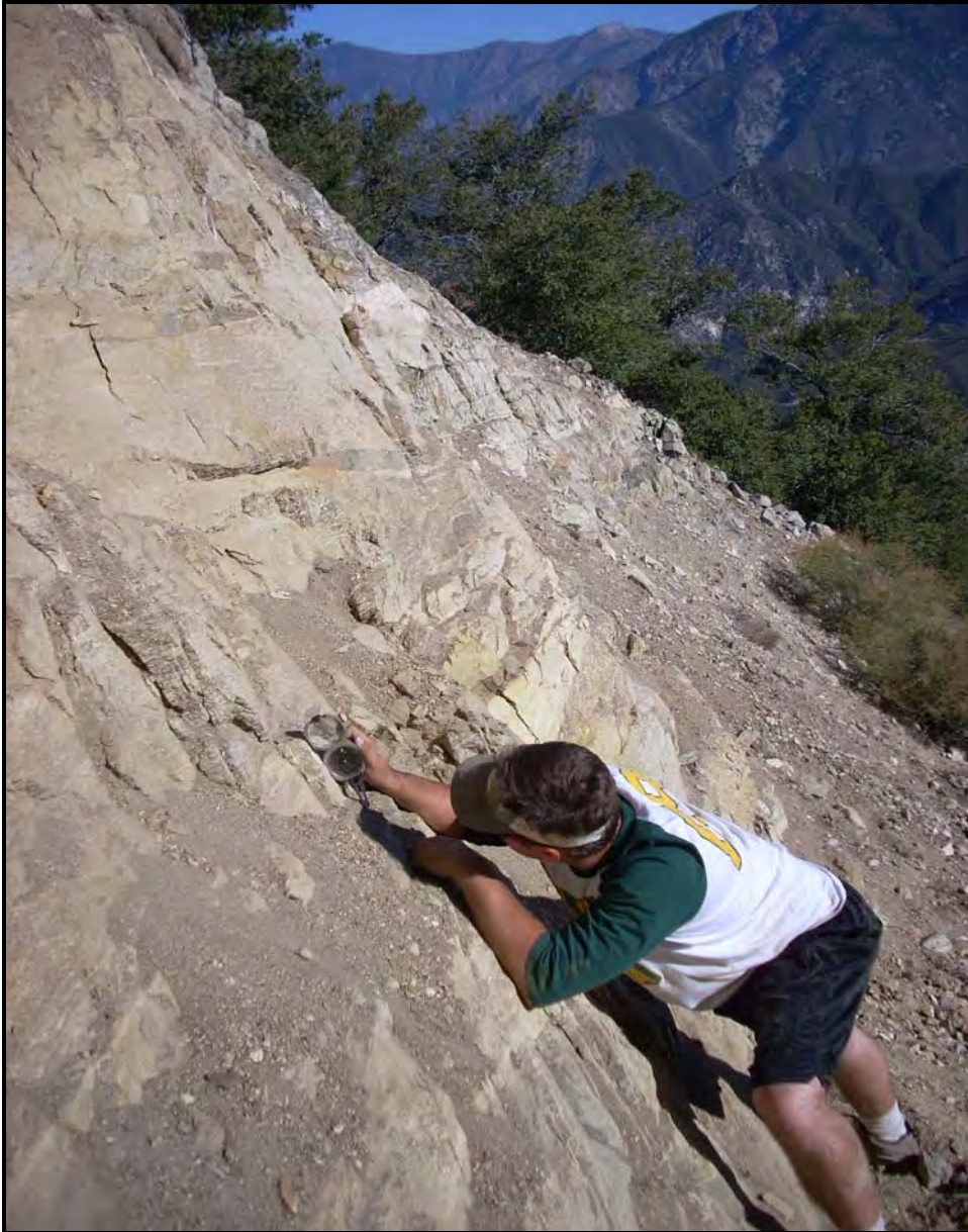
Figure 7. Measuring the steep dip of the back release surface. This is looking towards the North West.
