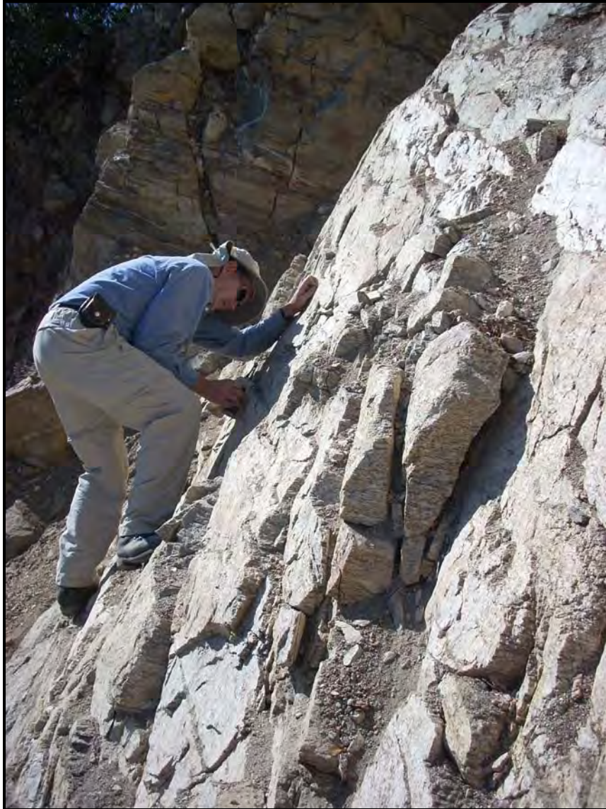
Figure 6. Taking strike and dip of a set of fractures oriented with the steep back release surface.
