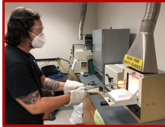
Melting rocks to make glass beads for XRF analysis
